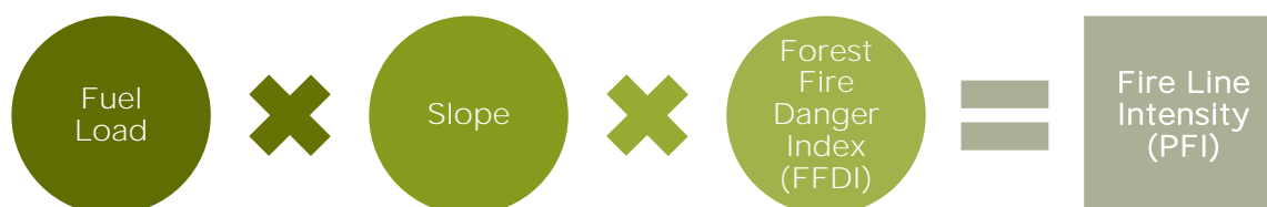
Figure 5: SPP Method for calculation of potential fire line intensity (PFI) (Leonard et al. 2014).
