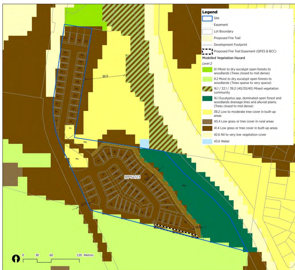
Figure 15: Separation between proposed lots and hazardous vegetation.
