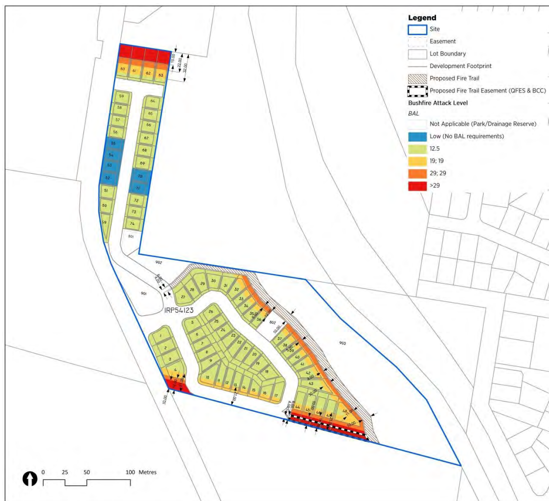
Figure 17: Bushfire Management Plan including Bushfire Attack Levels (AS 3959-2009).
